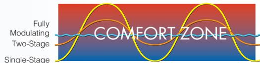
Your present furnace more than likely allows a temperature swing of 3° to 5°F before turning on or off. With an American Standard multi-stage gas furnace those days are gone forever.
